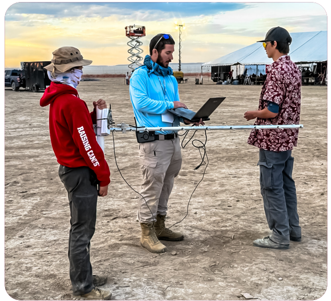
Figure 5: Antenna Testing at the IREC Competition to ensure a stable data link between the rocket and the ground.
