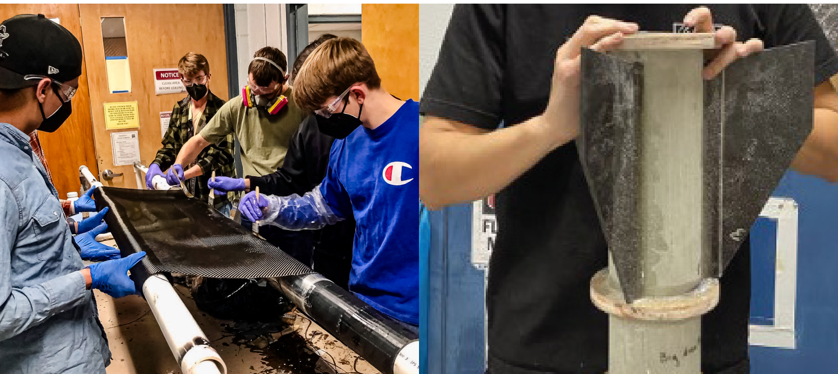
Figure 12: Rocket manufacturing wrapping the tubes and motor mount.
