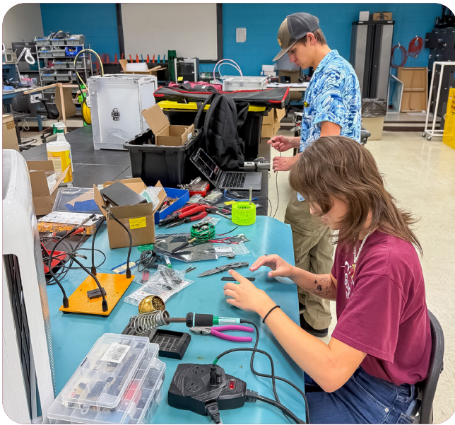
Figure 4: Fabrication of Version 1 Flight computer and telemetry system. Starting with custom designed Printed circuit boards and soldering on all necessary components.
